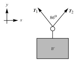
Decompose these tension vectors into components along the x- and y-axes. Because the resultant points directly upward and the tensions are equal, the angles from the vertical are  $43^{\circ}$ .
