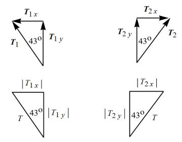
The corresponding triangles with the magnitudes are drawn as well. Use trigonometry to determine the vertical components.
